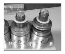
12) Place weep return rings (25) over the plunger (16) and pressure ring over plunger (24).
